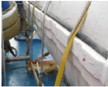
Figure 10: Incorrectly stowed life raft
