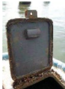
Figure 9: Hatch without a locking pin
